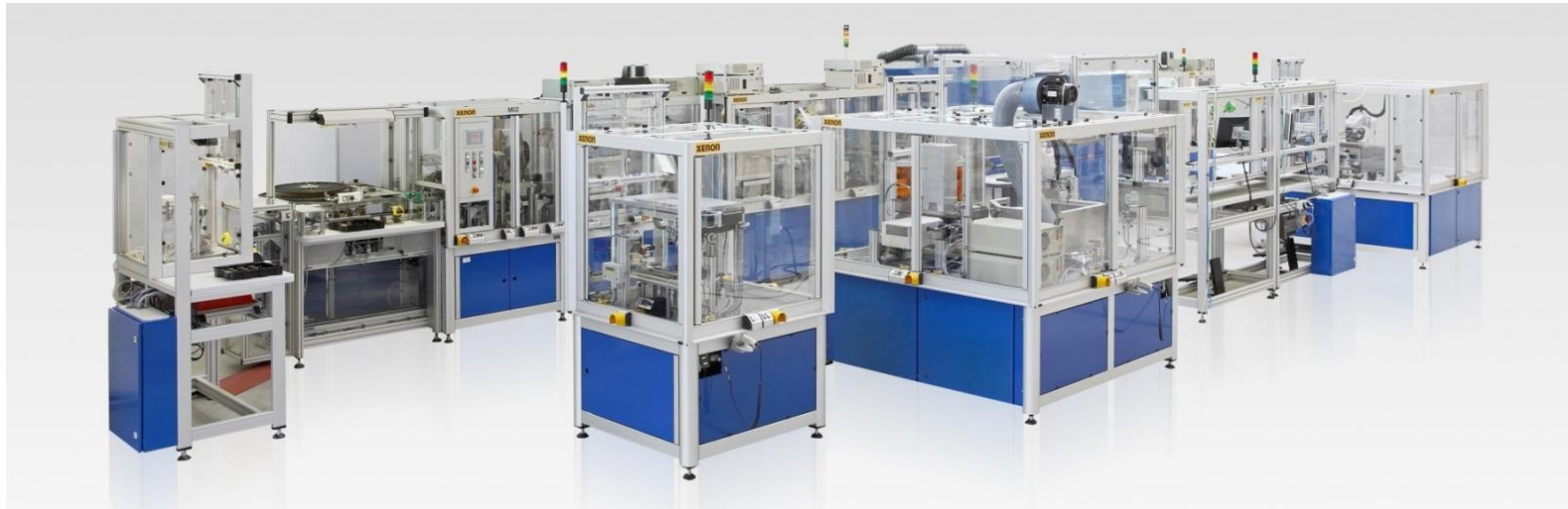
Production line for 3D-MID combi switches
